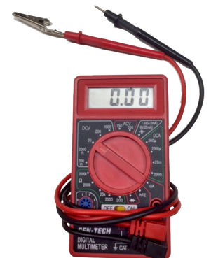
DVOM-Digital Volt Ohm Meter- Handy tool for diagnosing and measuring voltage, resistance and current.
