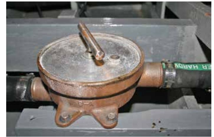
Fig 4 – Seawater strainer with removable top.
