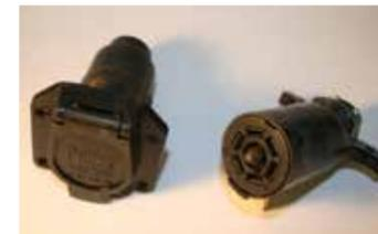
Figure 2: This is a Pollack heavy Duty spade or blade connector
