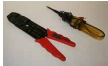
Figure 7: 12V Test light and combination wire stripper and lug crimping tool
