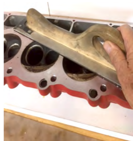
Figure 4 - A few strokes with long sanding board with 60 grit paper works well to remove the remaining bits of material from the surface after you first clean the surface with a razor blade scraper. This may also show some low spots.
