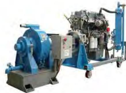
Fig. 2 The engine is typically mounted on a separate mounting cart which allows it to be wheeled into the test cell where it is attached to the dynamometer prior to testing.
