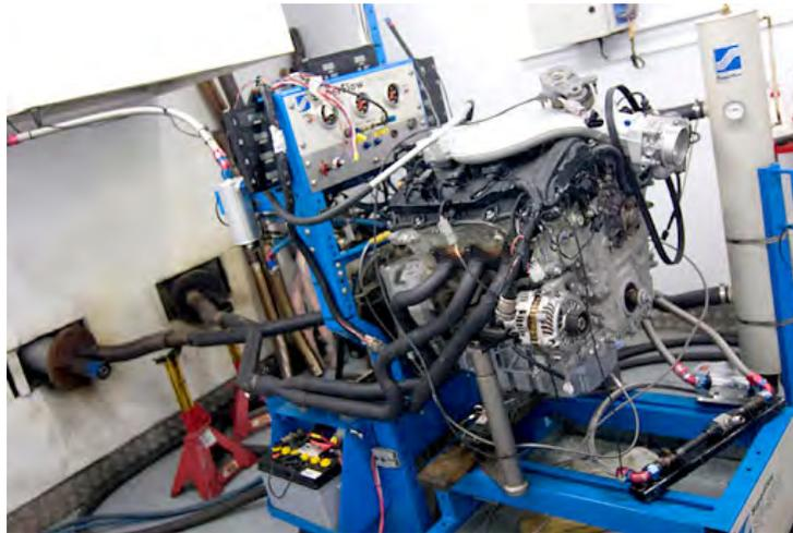
Fig.3. Dynamometers came in all sizes and with many features. The more expensive ones are electric and feature the ability to "motor" or turn the engine at speed without it running in order to measure the internal friction and pumping losses.
