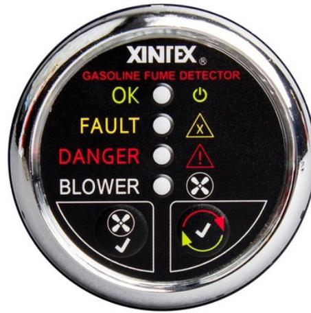
Fig 2 – This fuel sniffer will sound an alarm when it detects gasoline fumes, and then provides the option to automatically turn on the Bilge Blower.
