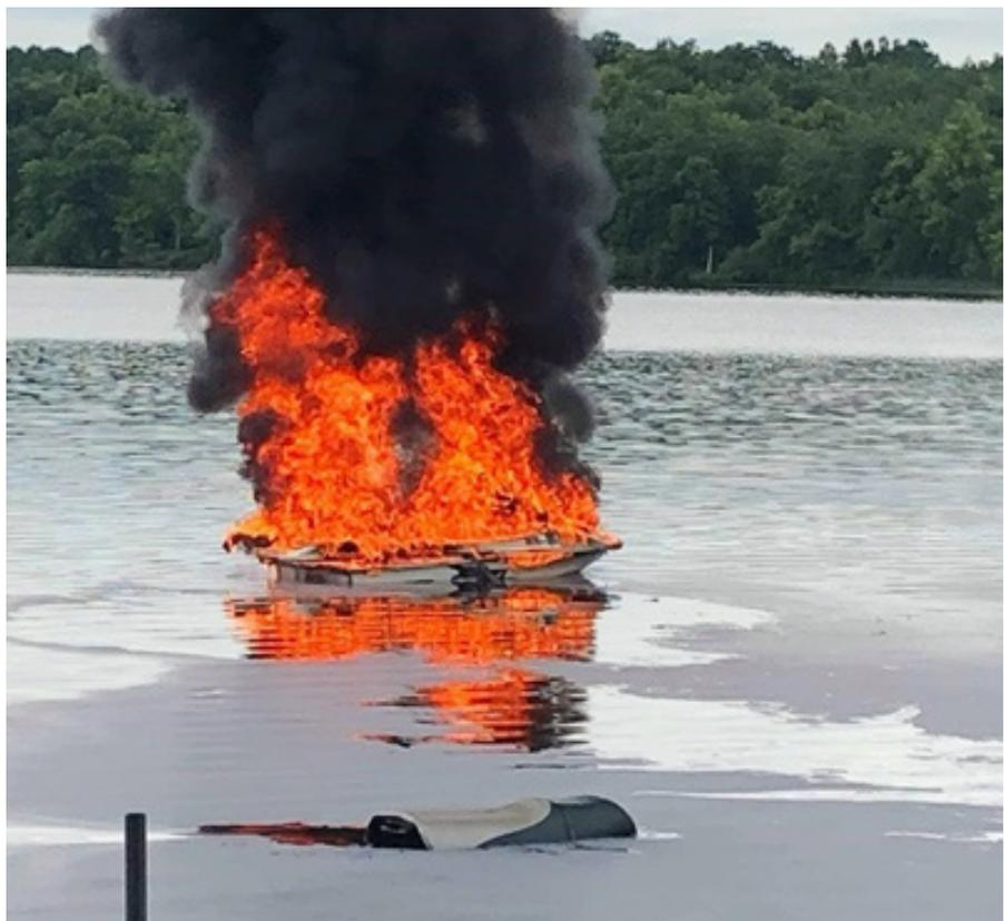
Fig 1 – Upon starting his jet ski, the individual was blown off his jet ski when leaking gasoline led to an explosion.
