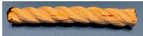
Fig. 2 – Three strand twisted nylon rope with a melted end to prevent unravelling.
