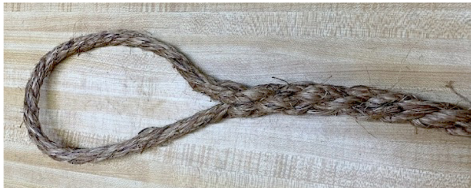
Fig. 1 – Three strand twisted Manilla Rope with a traditional tapered splice on one end.
