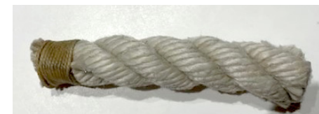
Fig.6 – Here we see the bitter end has been whipped with special wax coated string to prevent it from unravelling.
