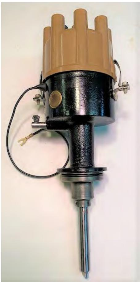
Using a football analogy, if the spark is the football, the distributor could be considered the quarterback of the engine team. Before a cylinder fires, the distributor sizes up the situation in the engine and then passes the spark at the right time and in the right place to make the most power. Before we begin our analysis, let's take a moment to suffer through another quick lesson on Internal Combustion Engine (ICE) operational theory.
