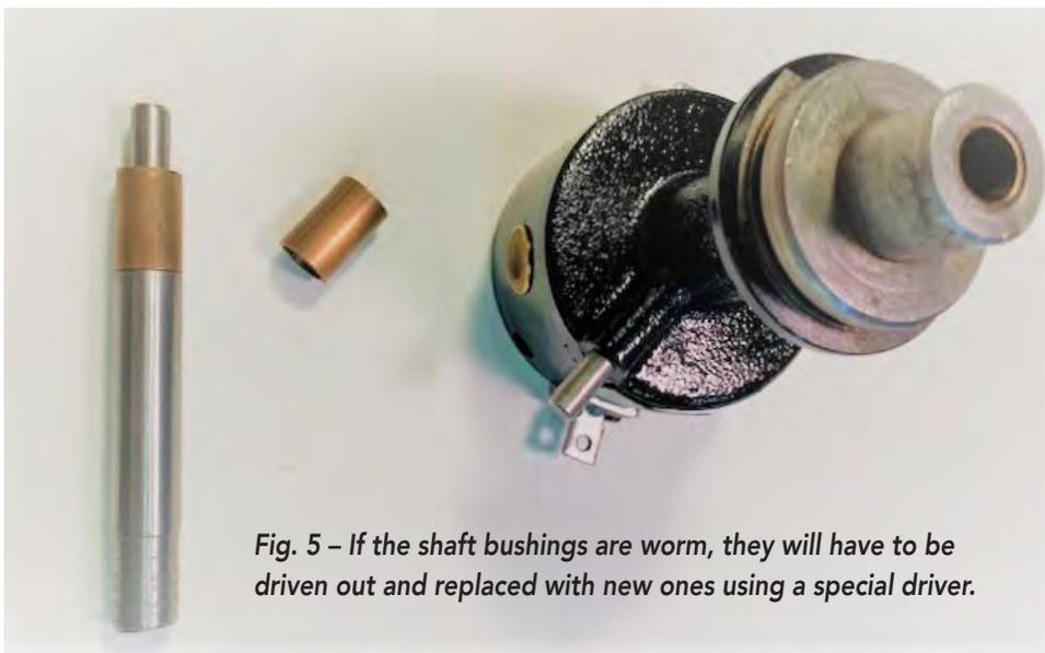
*Fig. 5 – If the shaft bushings are worn, they will have to be driven out and replaced with new ones using a special driver.*
