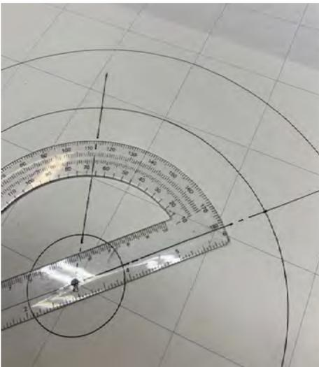
**Fig. 8 – Measuring the 67 deg. angle between the two lines formed by the upper and lower parts of the blade**
