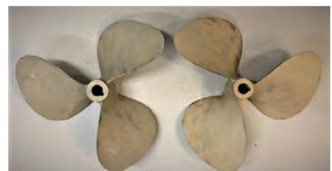
**Fig. – 4 The left-hand LH rotation prop is on the left while the right-hand rotation prop is on the right.**
