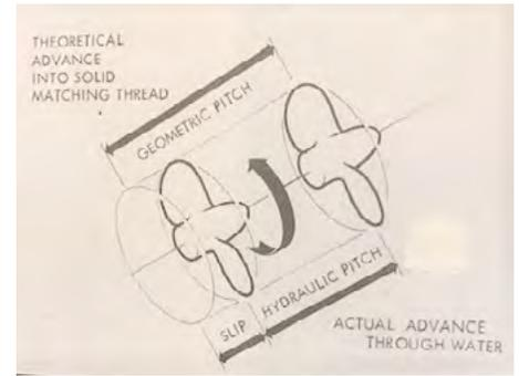
**Fig 3 – The hydraulic pitch of the propeller is the theoretical pitch minus the slip.**
