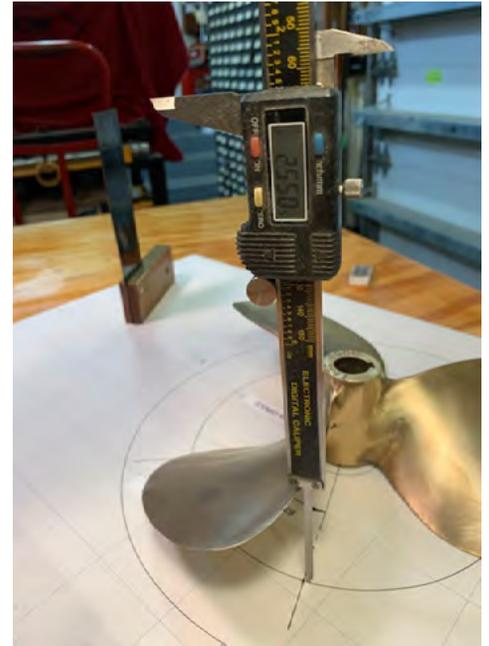
**Fig. 9 – Measuring the upper blade height on the pitch circle.**
