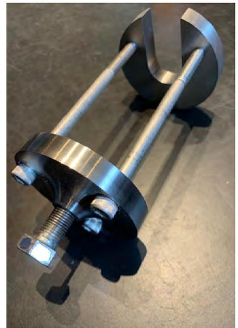
**Fig. 12 – A mandrel style prop puller that is less likely to damage the hub.**
