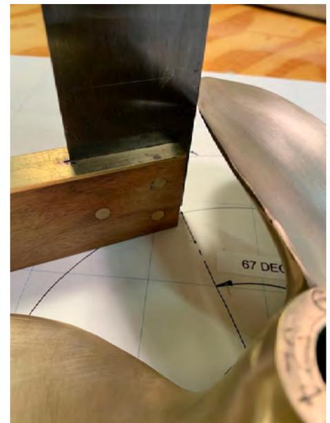
Fig. 6 – Place a square next to the blade and make a mark at the base of the square where it meets the pitch circle to locate a line.
