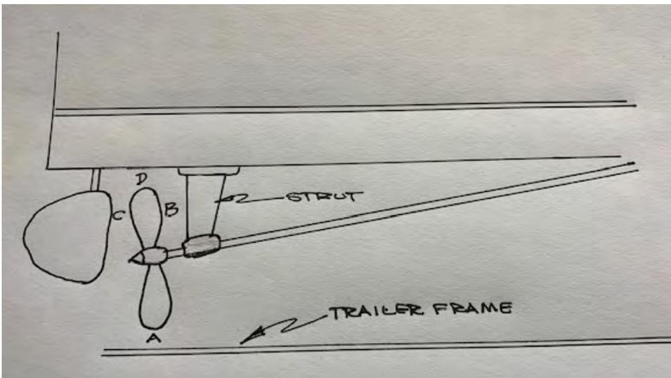
**Fig 2 – The propeller size is determined by the space available**
