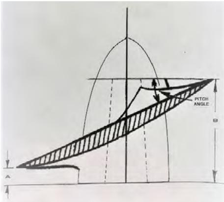
**Fig. 7 – The two height dimensions shown, plus the cross section airfoil shape of the blade at the pitch circle**
