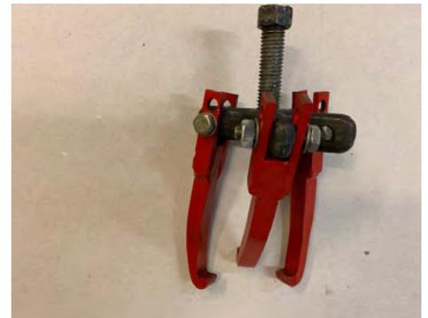
**Fig.10 – A three fingered prop puller**
