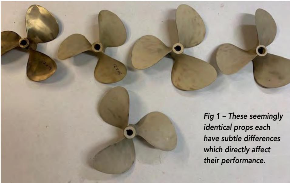
**Fig 1 – These seemingly identical props each have subtle differences which directly affect their performance.**
