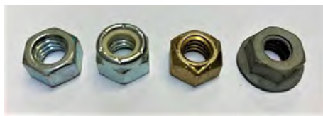
Fig. 8 – An assortment of nuts ranging L to R: a plain nut, a nylock nut, crimped or locking thread nut and finally, a standard flange nut designed to spread the load.
