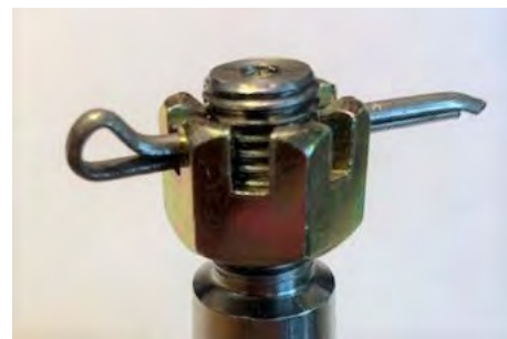
Fig. 9 – An assembled castellated nut with a cotter pin.
