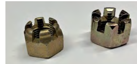
Fig. 10 – Two castellated lock nuts illustrating the difference between aircraft style on the left to automotive on the right. The tangs on the aircraft nut have been subtly machined to remove the excess material to save weight.
