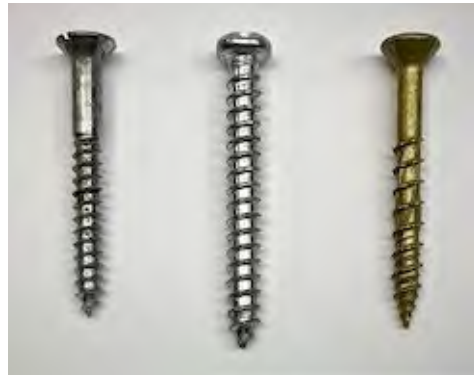
Fig. 1 – The wood screw on the left shows a defined shoulder while the sheet metal screw has threads over its entire length, and on the right, the drywall screw shows a coarse pitch thread.
