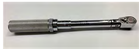
Fig. 8 – A torque wrench was the preferred method of establishing proper clamping load in fasteners until just recently when the torque-angle method has emerged as the preferred method for the newest class of fasteners.
