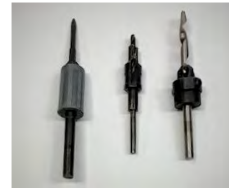
Fig. 3 – Special drills used for installing wood screws. The unique profiled shape creates a proper tapered hole with a countersink for the screw head thus ensuring good thread formation and maximum clamping load capability. Correctly adjusted, they take the guesswork out of drilling screw holes.
