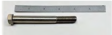
Fig. 6 – Shown here is a 4" fastener, where the length of a fastener is measured from the bottom of the head to the end of the threaded portion. Good practice suggests that an installed fastener should have at least three threads sticking out of the nut when properly installed, since the first three threads are usually smaller to aid starting and are therefore non load bearing.
