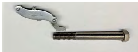
Fig. 7 – A thread gage available in either Metric or Imperial is used to determine the thread pitch.
