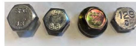
Fig. 2 – Material strength of Metric bolts is determined by the numerical rating indicated on the head of the fastener. Shown are fasteners with strength designations ranging from 4.8 through 12.9. 4.8 would be suitable for a screen door hinge while a 12.9 might be found on an aircraft landing gear assembly.
