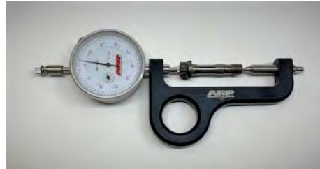
Fig. 6 – Stretch Gage used to measure rod screw stretch
