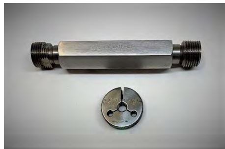
Fig. 7 – Go-no-go thread gages used to inspect and rank threads within a given size range.
