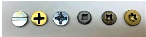
Fig. 2 – Various screw head configurations shown L to R the slotted screw, Reed & Prince, Phillips, square, modified square, and finally the Torx or star. While still used, the slotted head screw has been relegated to period correct restoration work. The other configurations have evolved due to their ability to speed production while reducing unintended disengagement. The square and Torx varieties have become popular as mechanical drivers have provided not only secure engagement but also increasingly more torque capability.
