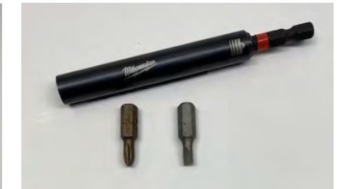
Fig.4 – Perhaps the handiest gadget I have used in a long time, this driver from Milwaukee Tools which accepts a variety of hex replaceable bits. It incorporates a sliding sleeve which slides over the head of the screw to guide and support and align the screw while it is being installed or removed. It prevents the driver from slipping out and ruining your varnish job!
