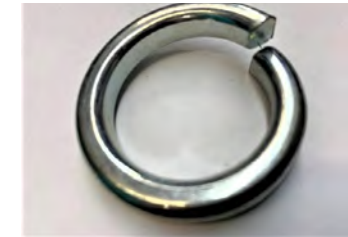
Fig. 12 – The lowly spring washer. Widely used but marginally effective and prone to break.
