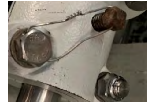
Fig. 13 – Safety wire used to prevent the prop shaft grub screw from loosening
