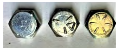
Fig. 1 – The strength of the alloy used in a standard Imperial fastener is typically indicated by the number of markings shown on the head. A low strength one without marking as shown on the left. The grade 5 with three marks is in the center while the strongest is the grade 8 with 6 marks on the right.
