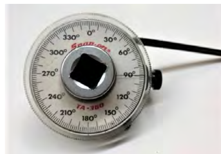
Fig. 9 – A torque-angle meter which when installed between a wrench handle and socket will indicate the angular travel.
