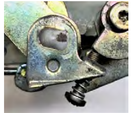
The choke idle screw controls the idle only when the choke is engaged. The screw is a bit difficult to reach so you will need a stubby screwdriver.
