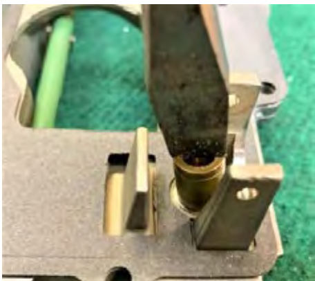
Step 6 – Notice how the float valve seats are mounted at an angle to the face of the airhorn. Be careful when starting the thread to prevent from cross threading.
