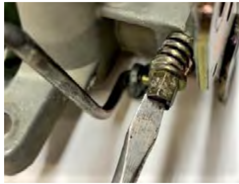
Idle screw. This sets the main idle when the engine is warmed up.
