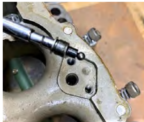
Step 9 – A magnet can be used to retrieve the accelerator check ball. This ball is held against its seat by a tiny brass weight.
