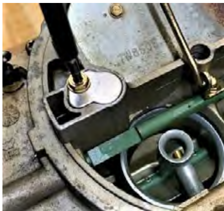
Step 2 – Remove the screws retaining the metering rod covers.
