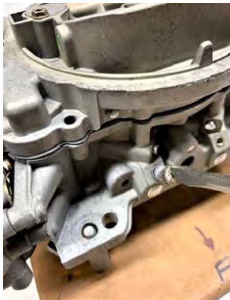
Step 10 – The main idle mixture screws
