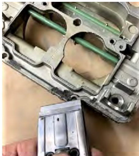
Step 7 – Use a razor knife to remove any small remaining pieces of gasket material.
