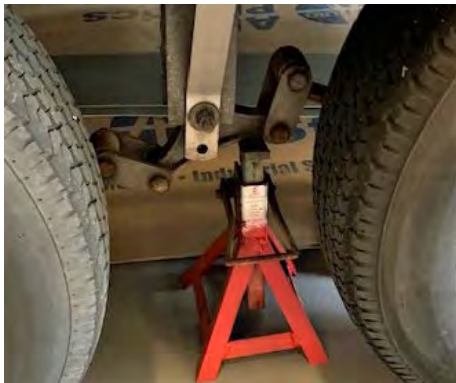
When working near or under a trailer or vehicle, always use a jack stand in case the jack fails.
