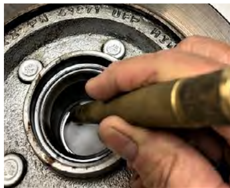
A brass rod is used to catch the inner edge of the bearing race so it can be driven out. Move back and forth around the inner perimeter tapping firmly. Do not stay in one spot to prevent cocking.
