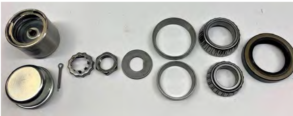
From left to right, the dust cover and Bearing Buddy followed by the cotter key Castle lock, and hub nut. The inner and outer bearing races and their matching bearings. Finally, the inner lip seal.
