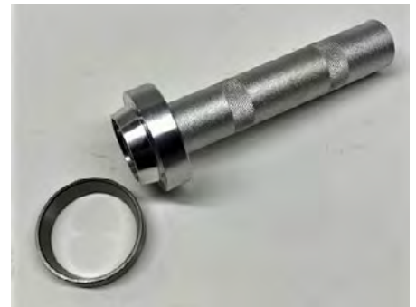
A bearing race driver. These make installing the new races in a snap, and they don't damage the race surface.
