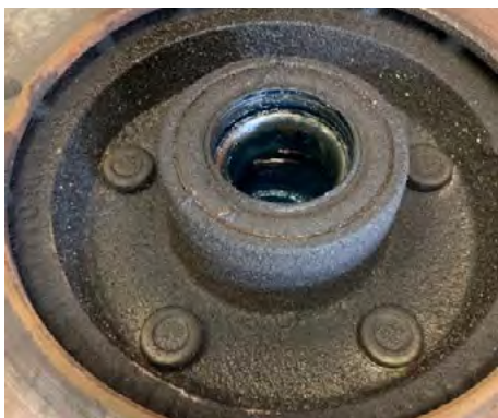
The inside of the hub and rotor assembly showing an overabundance of grease indicating a leaking inner seal.
