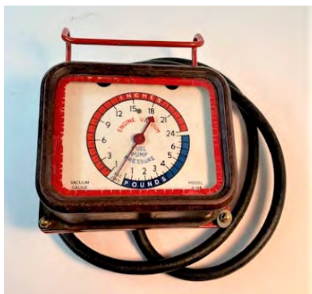
A combination vacuum-pressure gauge and inline tee fitting used to connect the gage to an existing fuel line. Useful in measuring not only fuel pressure which typically should range from 5-7 psi for a carbureted engine, but also able to measure intake manifold vacuum.
