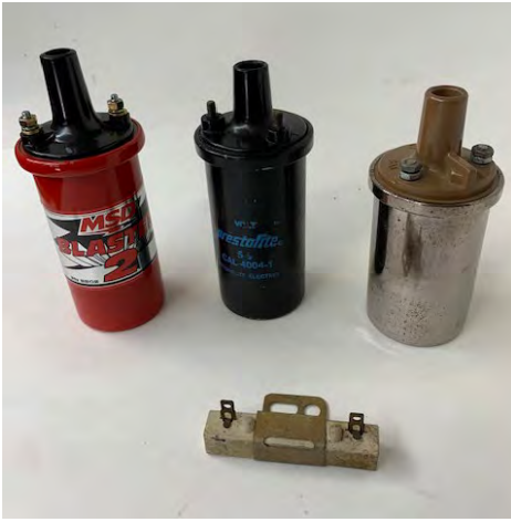
Ignition coils and a ballast resistor used to reduce the voltage going to the coil once the engine is running.
