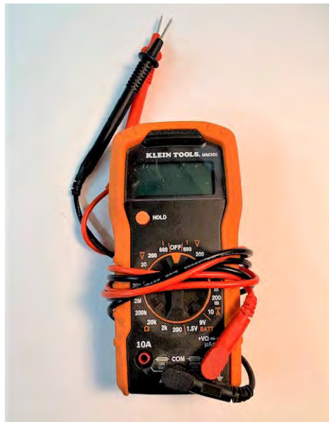
A Digital Volt-Ohm Meter DVOM. This is an essential diagnostic tool used to test voltage, resistance, as well as continuity.
