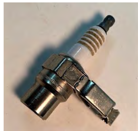
A test spark plug. Simply clamp to a grounded part of the engine and hook a spark plug or coil wire to the plug and see if there is a spark when the engine is turned over with the ignition on.
