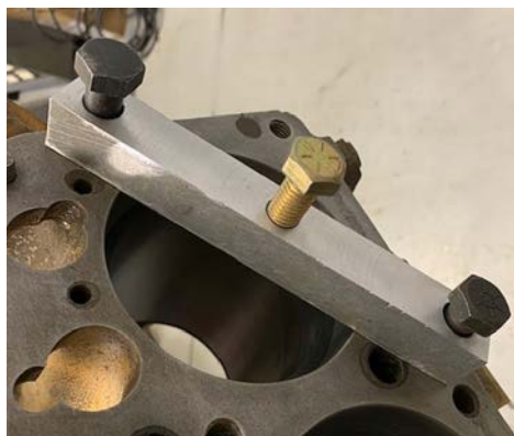
Fig. 15 – A solid bar appropriately called a hard stop is used to locate the piston at identical distances from TDC during clockwise and counter clockwise rotation. Half the distance between the two points is TDC.
