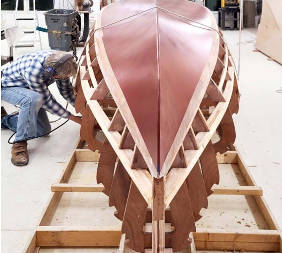
Completion of all laminations
