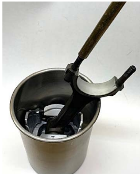
Fig. 12 – Prior to installation, dunk the piston rings and pin assembly in a container of oil and let it rest for a few minutes. This ensures that oil reaches all of the hidden areas and will be in place when the engine fires for the first time. Squirted oil on the rings and pin does not allow the oil to fully travel to the critical areas. Be sure to coat the rod bearing with oil before installation.
