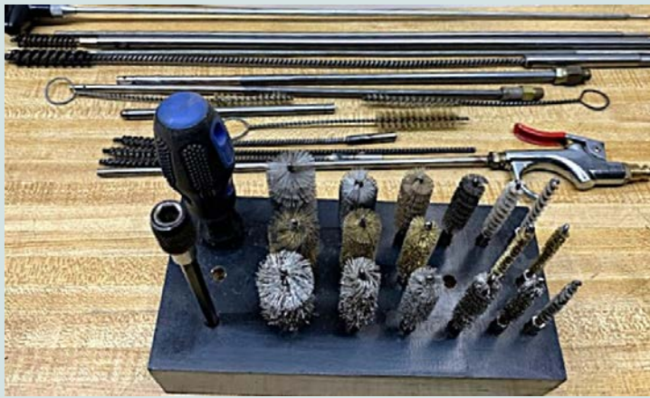
Fig. 4 – It takes an array of specialized brushes and extensions to properly clean all of the various oil passages correctly.
