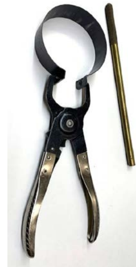
Fig. 14 – A ring compressor tool used to compress the piston rings during installation, and brass rod used to align and guide the rod while protecting the crankshaft.
