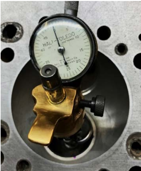
Fig. 1 – Hall-Toledo valve seat runout gage used to measure concentricity between the valve guide centerline and the valve seat surface.
