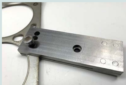
Fig. 16 – A special punch designed to punch accurate holes in metal head gaskets.
