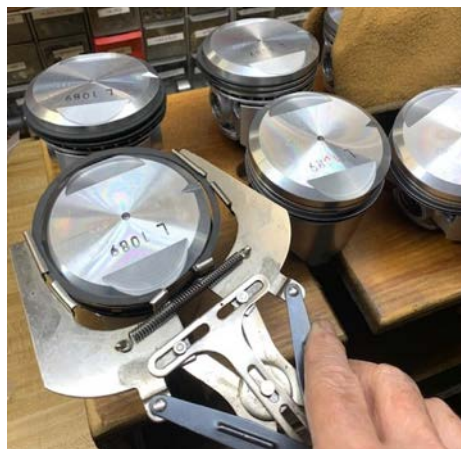
Fig. 10 – A special pair of pliers used to properly expand the piston rings allowing them to be installed on the pistons. Trying this without the tool is difficult and often results in a broken or damaged ring.
