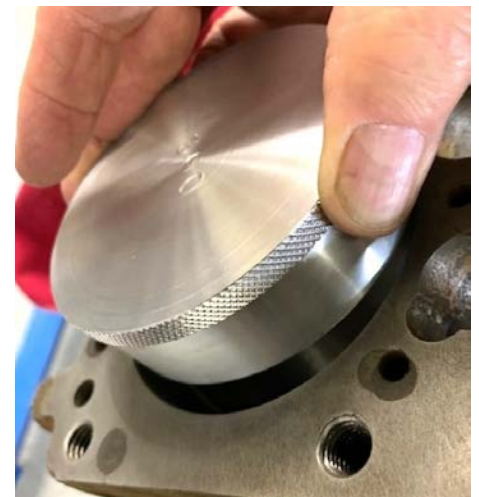
Fig. 6 – A special ring positioning tool is used to correctly locate each ring in its assigned bore so its end gap can be properly measured and corrected if necessary.
