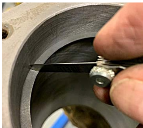
Fig. 7 – Once the individual ring is properly located in the bore, the end gap is measured using a small feeler gage.
