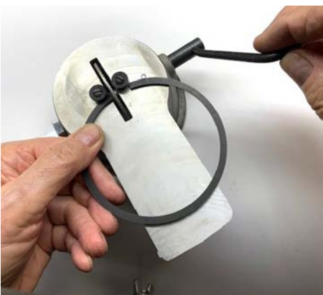
Fig. 8 – A rotary ring filer is used to ensure the ends remain perpendicular and parallel when enlarging the end gap.
