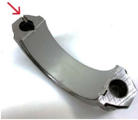
Fig. 11 – The oiling notch is shown with the arrow. Make sure the bearing and rod cap are clean and carefully slide the bearing into the cap. NEVER Scotchbrite™ the bearing surface to remove the coating. Bearings are covered with a special coating to prevent corrosion and enhance break-in.
