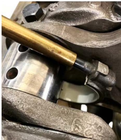
Fig. 13 – Brass rods placed over the rod bolts protect the crankshaft journal from scratches during assembly and disassembly. They are a good investment.
