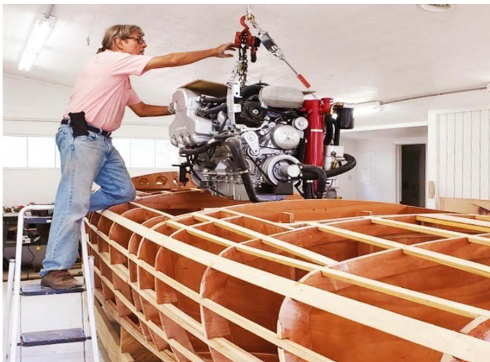
Temporary engine installation – with not an inch to spare!
