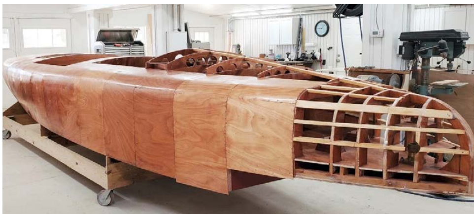
1st lamination of 1/8 inch Okoume plywood.
