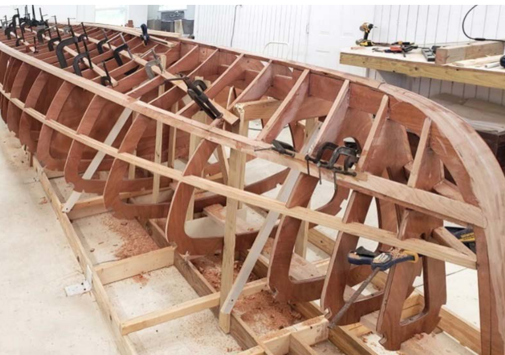
Frames and stringers completed.
