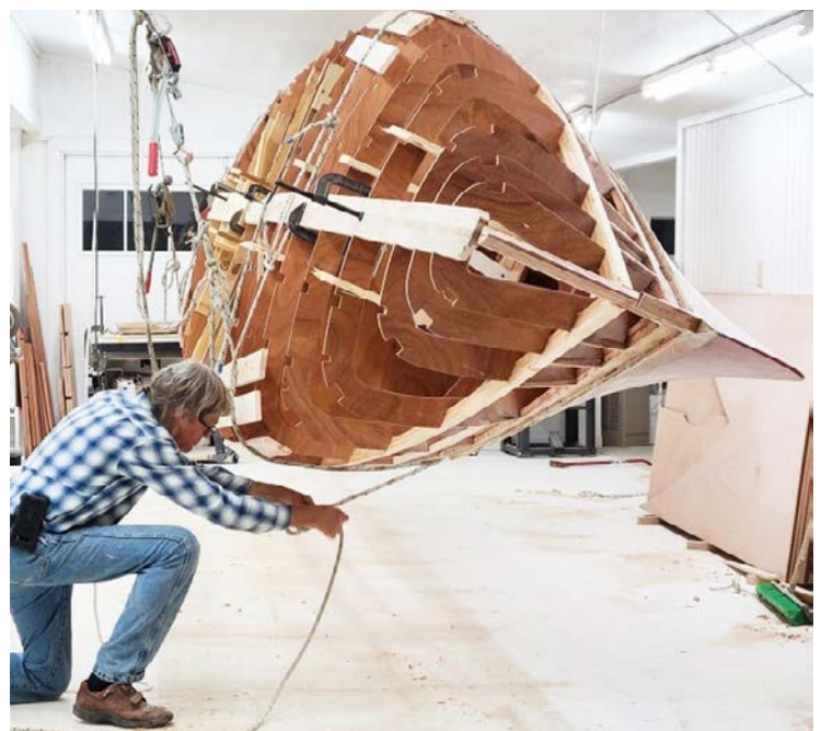
Jig removed – vessel almost upright.
