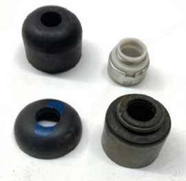
Various valve stem seals are available in many different shapes, sizes, and materials.
