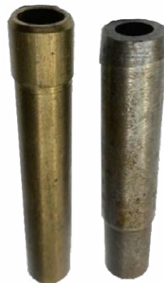
Replaceable valve guides are available in both bronze or cast iron.
