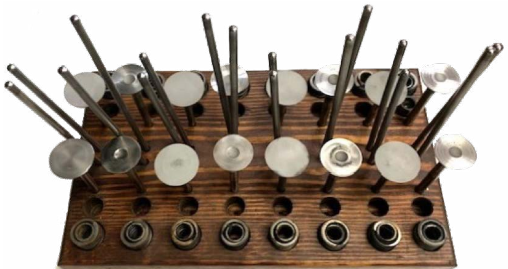
A valve gear board keeps all the individual components in proper order so they can be reassembled in their original positions if they are being reused.
