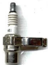
Fig. 2-A special test spark plug simplifies checking for spark. Attach the clip to a good ground and connect the plug wire.
