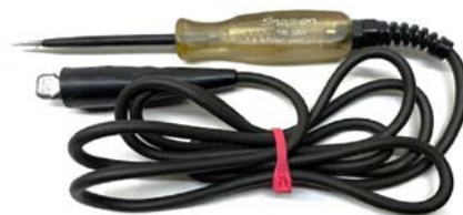
Fig. 4-A simple 12V test light quickly locates or confirms 12 volts. It's one of the first tools to have in your boat kit.
