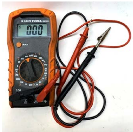
Fig. 5-A Digital Volt Ohm Meter accurately tests DC voltage, resistance in ohms, and continuity.
