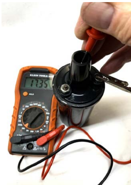
Fig. 7-Testing secondary winding resistance. The reading of 17.35 indicates a good secondary circuit.
