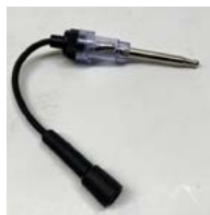
Fig. 3-Another tool, an inline spark plug tester, makes testing for spark easier.
