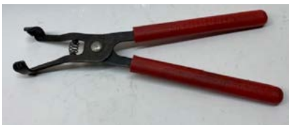
Fig.1 – Special insulated spark plug wire pliers make grabbing a hot, high-voltage wire near the exhaust manifold easy. Once you use them, you won't return to the bare-handed method.
