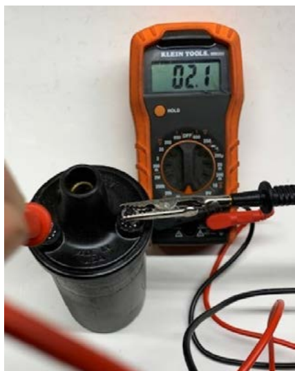
Fig. 6-Testing resistance between the positive and negative terminals of the primary winding circuit.
